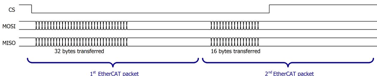
For example, a transfer of 48 bytes would be split across two EtherCAT packets. This happens transparently to the Host except that the transfer would take one extra millisecond to complete, and so reduces the maximum number of transactions per second to 500.
